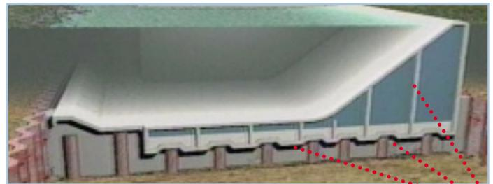
Cast-in-place SLC interior supports and floor sections
