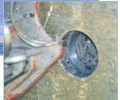
Core samples reveal lightweight aggregate concrete has held up very well in extremely harsh marine conditions.
